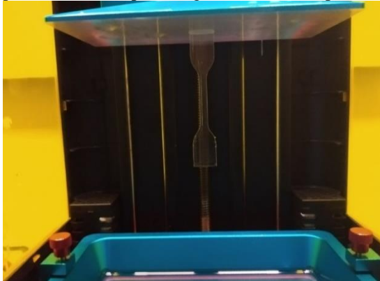
Fig. 11. One sample on build plate
