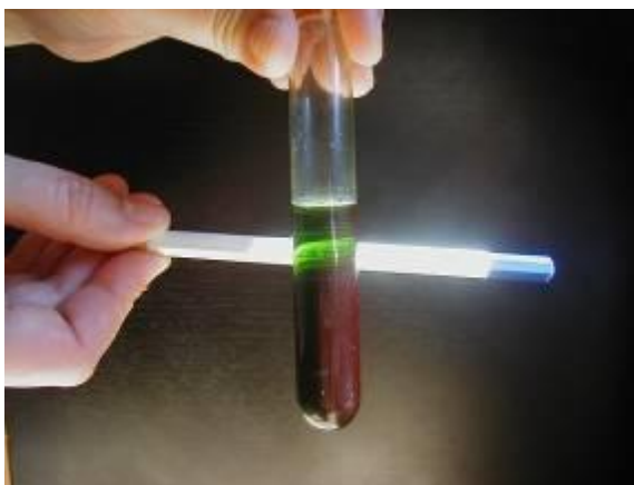
Fig. 8. Observing fluorescence in solar light. The entire sample tube is red, excepting area observed by transparency which is green
