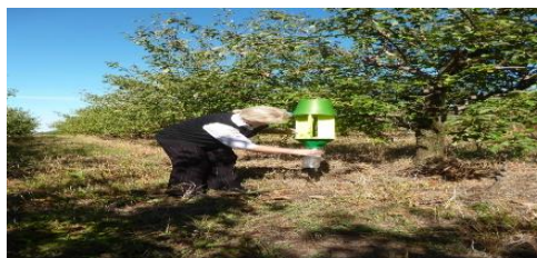
Fig. 2. UV trap irradiation for orchard pests control.
