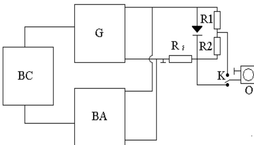
**Fig. 1. Electrical scheme for measuring the electrodynamic characteristics of the pulse electrical discharges (BC- controll block, G – pulse generater, BA initiating block, O – oscilloscope,  $R_s$  – electrical shunt , R1 – R2, voltage divizor, K – commutator**
