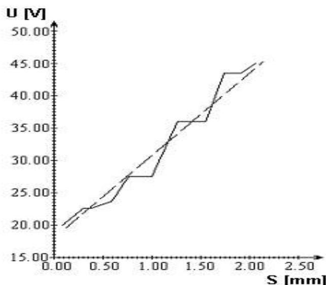
**Fig. 2. The influence exerted by the gap size on the voltage in the gap**
