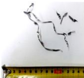
v_c = 73 m/min, f_z = 0.052 mm/Zahn a)
