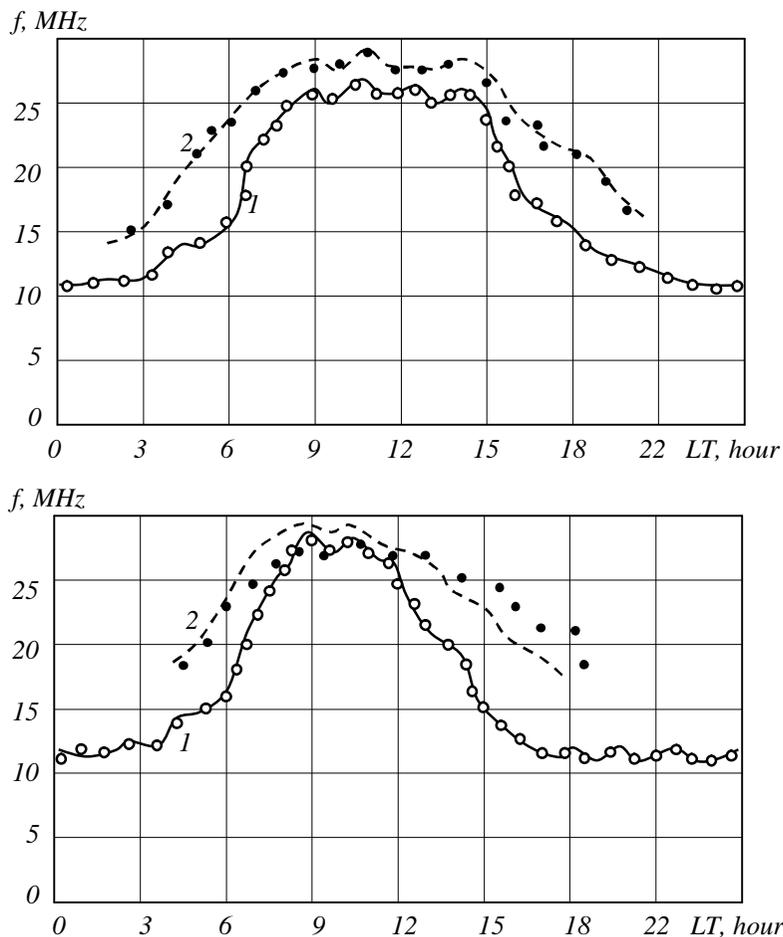
Fig. 5. (a) Diurnal variations of maximum observed frequencies:  $\circ$  – control trace Dushanbe-Bălți (experiment),  $\bullet$  - work trace Dushanbe-Kiev (experiment); by 1 is denoted the corrected prediction of maximum observed frequencies using data of the oblique sounding for the trace Dushanbe-Bălți, by 2 is denoted an extrapolation of maximum observed frequencies from the control route to the work trace Dushanbe-Kiev.
