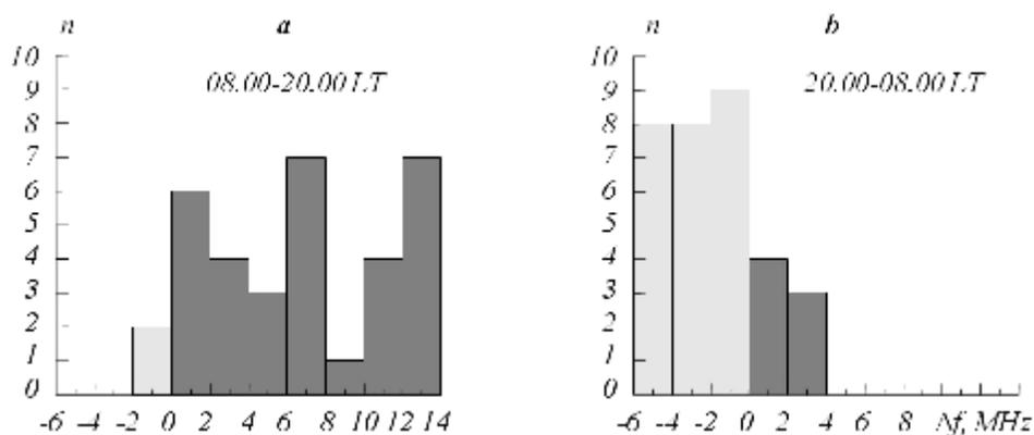
Fig. 1. Histograms of distribution of frequency difference of the related signals,  $\Delta f = f_1 - f_2$ , selected by knowledge of the long-term ( $f_1$ ) prediction and short-term ( $f_2$ ) prediction for diurnal (a) and nocturnal (b) hours [3].
